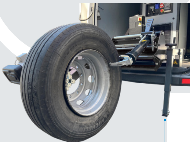
megamount 2-26T2 : model with right-hand chuck orientation
